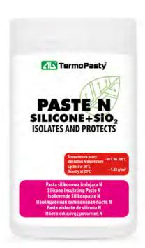
A silicone paste that effectively isolates and protects from atmospheric influences. The product protects from ground faults, preserves rubber, plastics, and what is important, it has a wide operating temperature range from -40°C to 200°C. It is characterized by a very good chemical resistance to oxidation, the effect of aqueous solutions of acids, alkali and salts, sulphur dioxide and ammonia.
