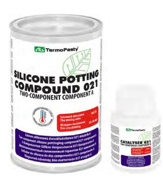
The product is a liquid filling, two-component material. Hardening occurs at a room temperature. The material provides thermal conductivity and low expansion. Ideal for pouring or filling joints in heatgenerating electronic components with metal housings or radiators. It has an excellent fluency at dosing and filling. After hardening, it does not tear off as a result of cyclic heating from a surface, to which it is attached. Hardened product is dry to the touch.
