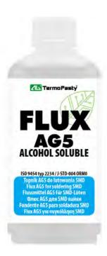
A liquid, rosin-free, medium-active fluxing agent (ISO 9454 typ 2234 / J-STD-004 ORMO), which is an alcoholic solution of organic compounds. Used for high temperature (300-400°C) tinning and soldering of elements coated with polyurethane varnish and soldering silver-plated and tinned elements.
